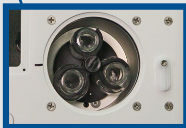
Refrigerated compartment for 3 vials of Lyophilized Bacteria
