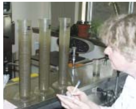
In the traditional 30-minute sludge settling test, Water Quality Specialist Sarah Collins at the Renton, WA, wastewater treatment plant must manually measure and record blanket levels and construct a settling curve to identify sludge volume and sludge volume index.
